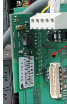
*Tarjeta receptora radio HF*
